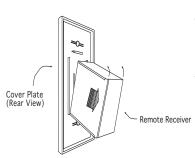
Position the receiver as shown in diagram to the left with lower tab on cover plate inserted into groove of receiver (Make sure LEARN hole on cover plate properly aligns with remote receiver). Pull receiver up and snap into top tab of cover plate.
