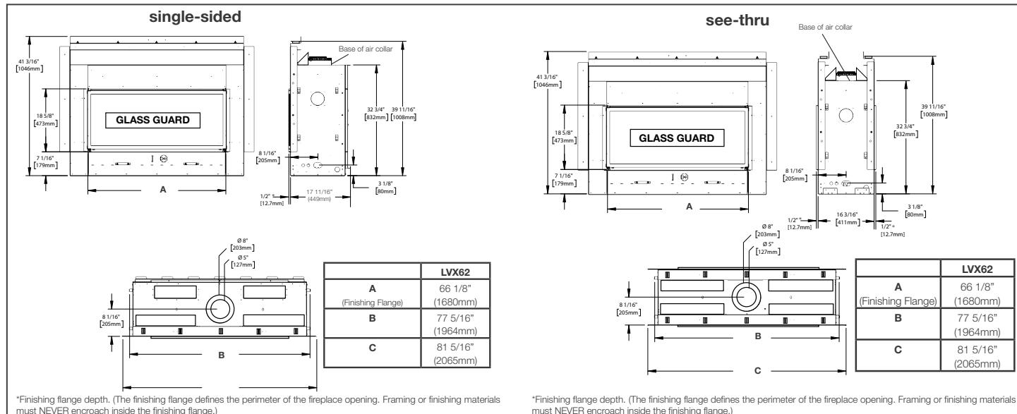
\*Finishing flange depth. (The finishing flange defines the perimeter of the fireplace opening. Framing or finishing materials must NEVER encroach inside the finishing flange.)
