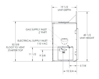
Caution: The distance from floor level to the centerline of the vent cap is based on Simpson DuraVent GS components. If using vent components of another brand, do not assume that the measurement given here is applicable. Verify the distance to the centerline of vent cap by measuring the components you are using.
