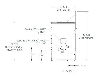
Caution: The distance from floor level to the centerline of the vent cap is based on Simpson DuraVent GS components. If using vent components of another brand, do not assume that the measurement given here is applicable. Verify the distance to the centerline of vent cap by measuring the components you are using.
