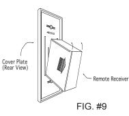
Position the receiver as shown in diagram to the left with lower tab on cover plate inserted into groove of receiver (Make sure LEARN hole on cover plate properly aligns with remote receiver). Pull receiver up and snap into top tab of cover plate.
